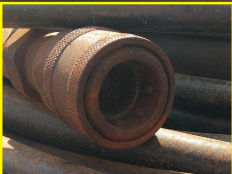
Corroded hydraulic coupling!
