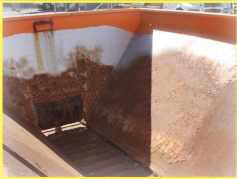
Spreader box corrosion!
